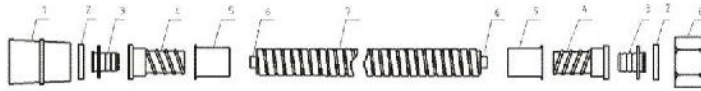
1- Brass nut with oring 2- Rubber 3- Brass insert 4- Plastic insert 5- Stainless Steel bell 6- EPDM inner tube 7- SS hose 8- Brass nut
